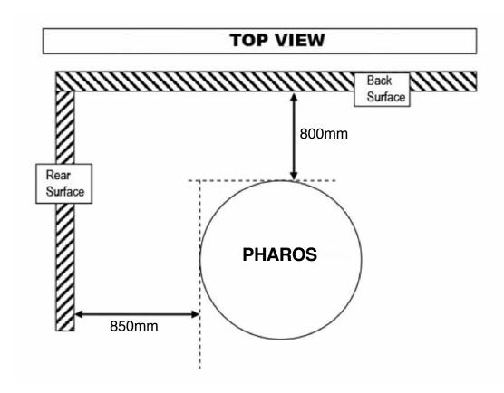
It is possible to reduce these clearances by installing heat shields between the unit and the combustible material. Installation of such heat shields has to be made in accordance with the BCA (Building Code of Australia)
